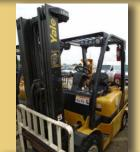
YALE 2006 GLP050VX, 5000# CAPACITY, SIDE-SHIFT, FFL 3 STAGE MAST 90"/200", B/U ALARM, LP 4636 HRS
