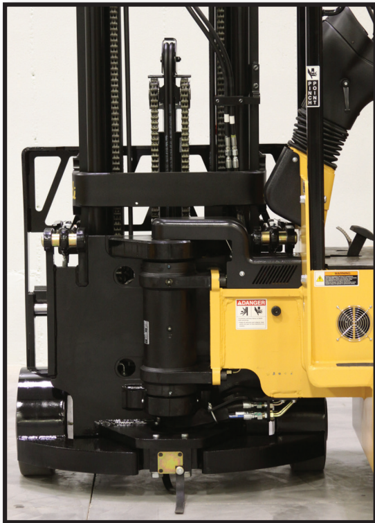
DuraSteer™ Front Wheel Steering *Patented
