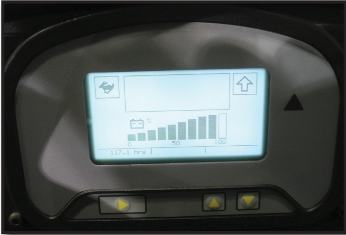
Dash Display with Full Diagnostics Battery Discharge Indicator and Hour Meter
